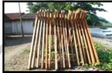
Figure 1. Vertically drying of wood
