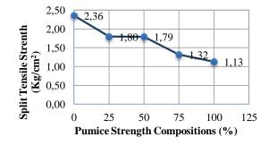
Figure 5. The relationship of split tensile strength with pumice sand composition as a partial substitution of fine aggregate
