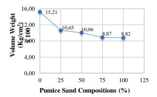
Figure 3. The relationship between volume weight with the composition of pumice sand as a partial substitution of fine aggregates
