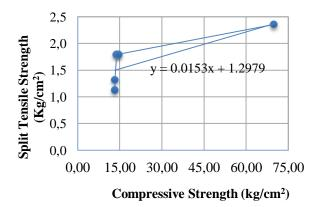
Figure 6. The relationship between split tensile strength and compressive strength with pumice sand composition as a partial substitution of fine aggregate
