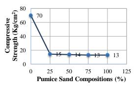
Figure 4. Compressive strength relationship with pumice sand composition as a partial substitution of fine aggregate
